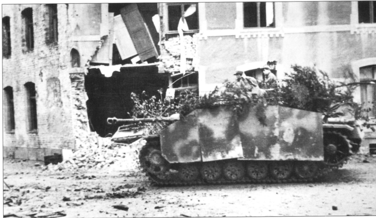
Above: A Sturmgeschütz assault gun of the Panzer Lehr Division fitted with Schürzen (side skirts) to counter shaped antitank charges. During the later stages of the war, German armoured vehicles received a coating of Zimmerit paste as a defence against magnetic charges.
