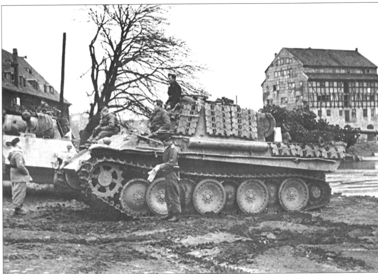
Above: A MkV Panther with spare tracks wrapped around its turret. The Panther was the German response to the Soviet T-34 and copied the former's sloped armour. After suffering serious teething problems in 1943, it acquired a formidable reputation; some 5500 were built.
